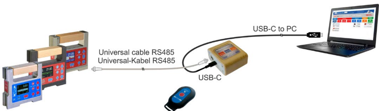
Connect wylerLEVEL / wylerCLINO to a PC using a cable connection via wylerCONNECT
