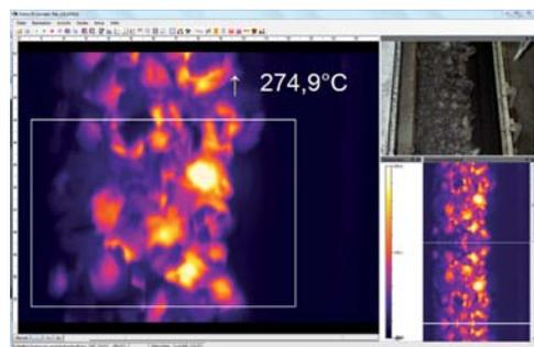
**Cross fading mode:** Highlighting of critical temperatures by cross-fading (0–100% transparency)
