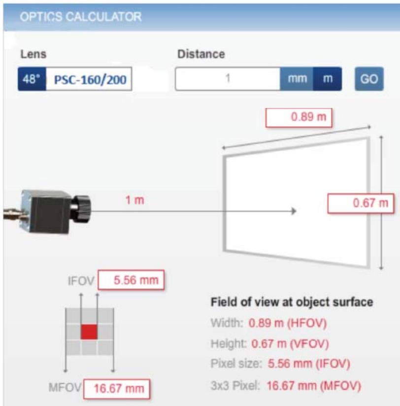
Lens of the thermal imaging camera determines the overall area of measurement displayed as a rectangular field of view
