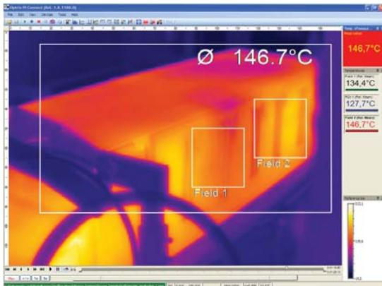
PSC Camera Connect, the user-intuitive menu-driven real time software sets new standards with its simplicity, versatility and functionality. The unlicensed and unrestricted software allows the operator to combine variable points with crosshair targeting and programmable areas of measurement with automatic displays of maximum, minimum or average temperature readings within assigned areas with multiple, user selectable regions of interest (ROI's).
