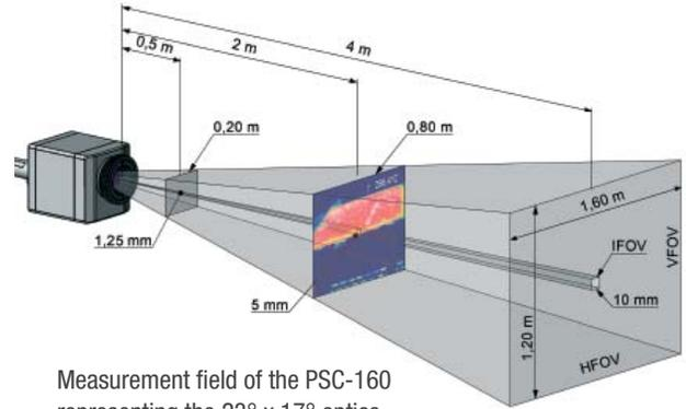
Measurement field of the PSC-160 representing the 23° x 17° optics.
